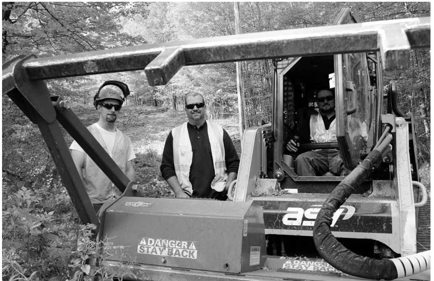
Lineworkers Eddie Wallace, Jamie Dailey, and Pat Morrissey (seated) with the trackloader with forestry head. "It's got a lot of torque to it, but it doesn't kick debris as far," as other forestry equipment, noted Rick Stergas.
