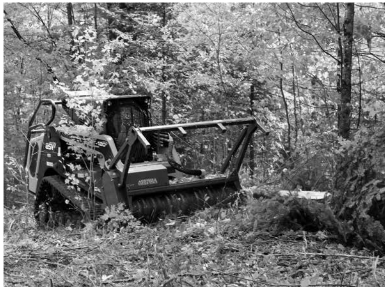
Pat Morrissey demonstrates how the machine demolishes vegetation in rights of way. Here, he pushes into a balsam, mows it over, and shreds the stump. Crews are interested to see if pulverizing stumps slows regrowth.
