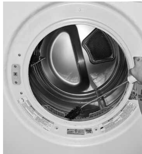
A step beyond the lint screen: a dryer brush catches and removes lint build-up. Too much dryer lint can be a fire hazard.
