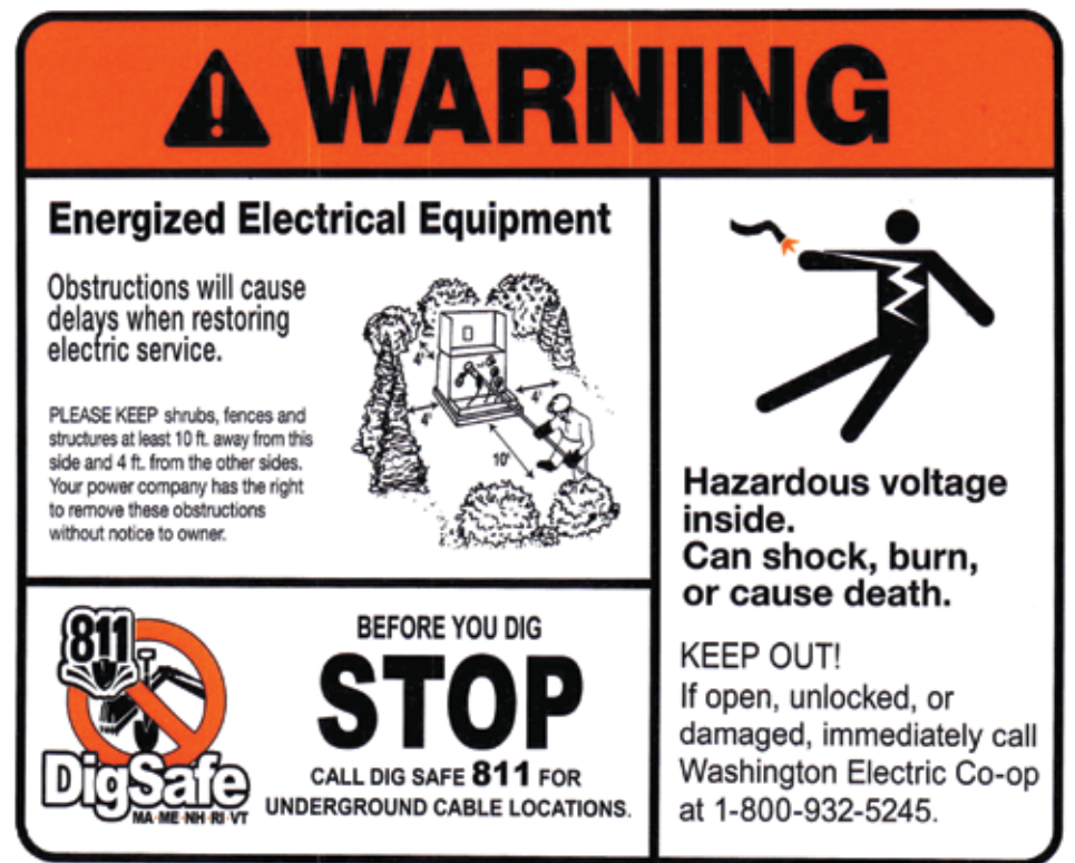
This warning sticker should be located on all padmount transformers.
